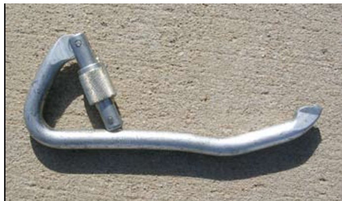
A General Use carabiner that was inadvertently tri-loaded during a slow pull test of an anchor sling. The failure occurred far below the rated capacity of the carabiner.
