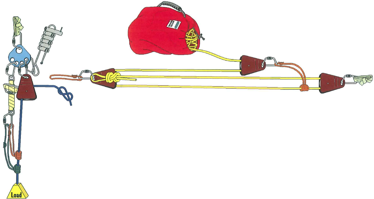
Figure 11-28: Construct 5:1 Pig Rig
