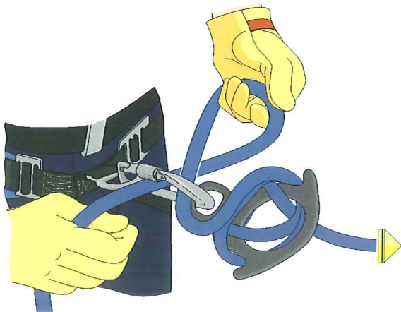
Figure 10-35: Twist the Bight Clockwise
